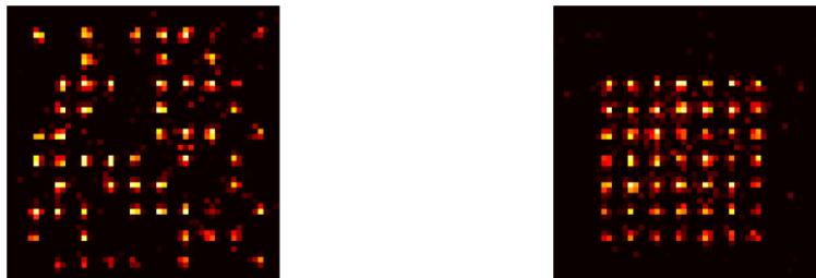
Figure 1 : Atom assembly of an atomic array (before / after). This technique, together with the excitation of atoms to Rydberg states, allows the simulation of spin models on systems of various geometries and size.
