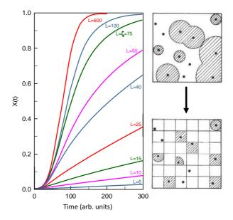
2-Dimensional simulation of the time evolution of the transformed fraction X(t) for different grain sizes (from above to below  $\xi$  ).
