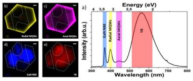
electron microscopy and then by X-ray excited optical luminescence and X-ray Fluorescence with multimodal hard X-ray nanoprobe [8]. It is shown that the optical luminescence of the near band edge of the GaN core is directly related to differential Si incorporation in N- and Ga-polar parts of thick wires, and that core-shell and top axial MQW luminescence can be analysed.
