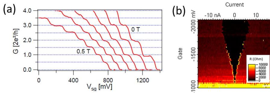
**Figure 1:** (a) Conductance measurement versus gate voltage of 1D ballistic Ge hole gas under out-of-plane magnetic field. (b) Resistance measurement of Ge JoFET versus current and gate voltage showing a superconducting transition.
