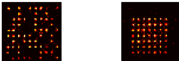
Figure 1 : Atom assembly of an atomic array (before / after). This technique, together with the excitation of atoms to Rydberg states, allows the simulation of spin models on systems of various geometries and size.
